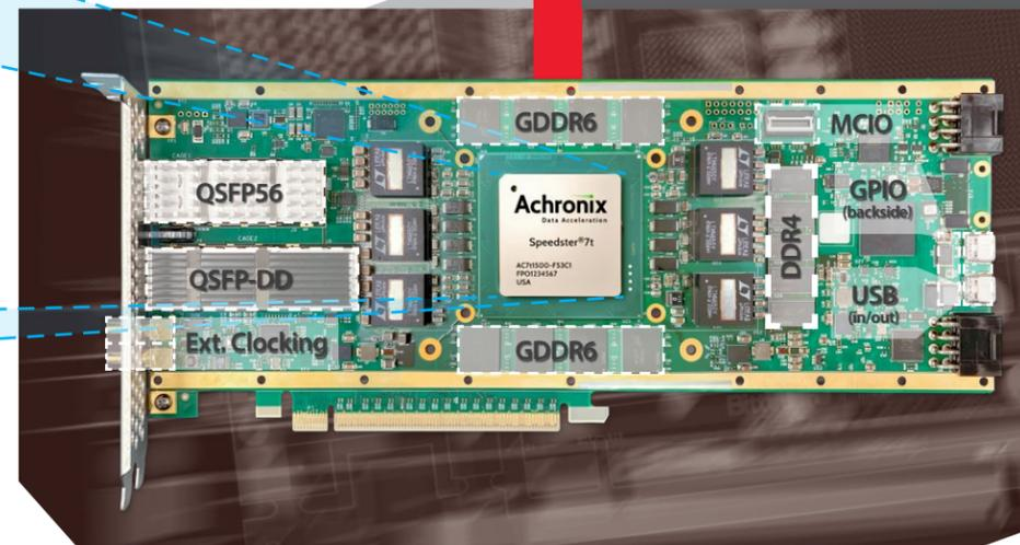
Unlocking the Speedster7t FPGA's potential is BittWare's S7t FPGA card, designed for both development and at-scale deployment. The S7t FPGA card delivers a wide range of advanced I/O, including 400G and multiple PCIe interfaces and the high-bandwidth GDDR6 memory. Customers can get started quickly with the BittWare SDK, including an example project, for Linux and Windows.
