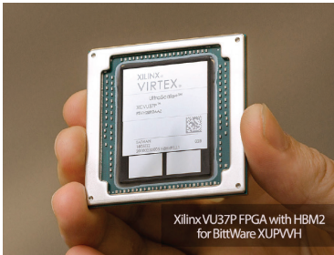
AMD VU37P FPGA: lidless package is used by BittWare's Viper thermal management for enhanced cooling performance
