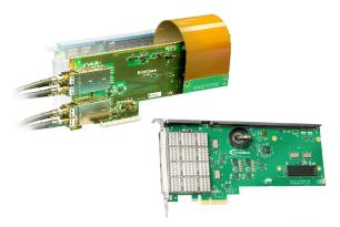
Optional accessory boards provide customization options such as x16 PCIe, 4x 100G, or video transceivers.
