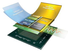
With 200 Gbps of digital I/O available on the FPGA side of the RFSoC, the card supports twice the bandwidth of RFSoC implementations that depend upon PCIe for data transfer. This I/O is available through two QSFP28 ports. Customers have implemented transports using Aurora, Ethernet MAC frames, and UDP.
