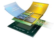
The AMD Zynq® UltraScale+™ RFSoC integrates RF-class A/D and D/A converters into the Zynq® FPGA fabric and multi-core ARM processor subsystem, creating a multi-channel data conversion and processing solution on a single chip.
