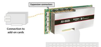
Integrated into custom server with front-port expansion breakouts
